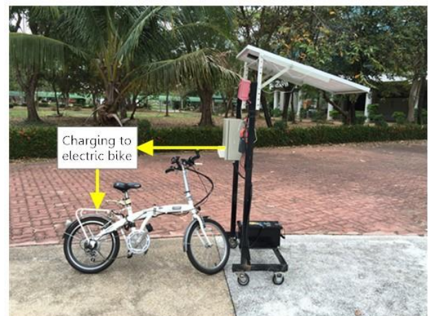
Fig. 10. Demonstration of electric bike parking and charging to solar PV mobile charging station.
