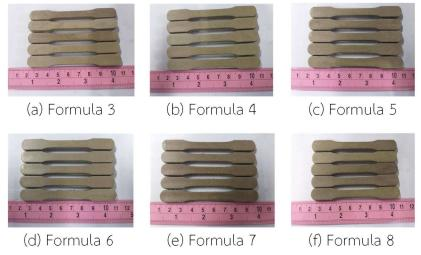
Figure 4 Green parts with different mixture ratio.
