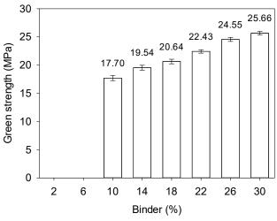
Figure 6 Green strength from three-point bending test.
