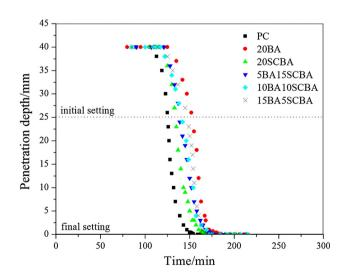
Fig. 2 Setting time of ordinary Portland cement containing BA and SCBA
